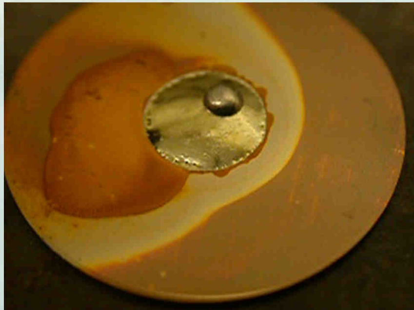
Poor Oxidation Barrier
