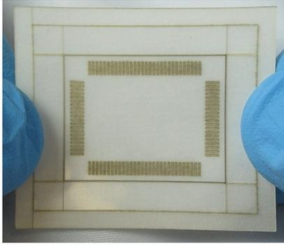
**STEP 1** Examine the stencil to make sure that it fits the land patterns on the PCB. Make sure site is wicked (if reworked) and cleaned.
