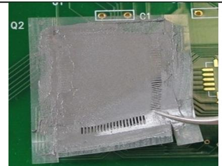
**STEP 7** Pull off the stencil carefully making sure no solder paste is accidentally smeared on neighboring areas of the board/parts. Discard stencil.
